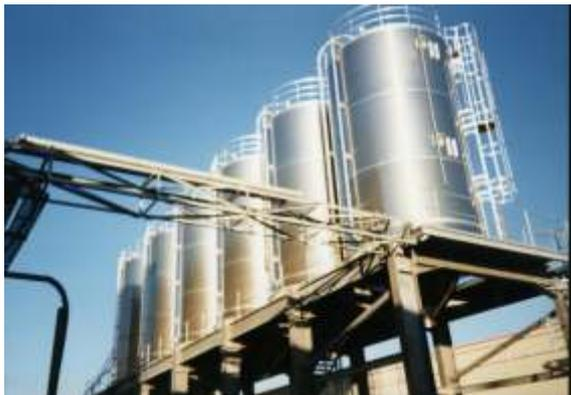
For high usage materials delivered to site by tanker or lorry we can offer bulk storage silos of varying capacity suitable for holding a variety of materials. Such storage facilities can be loaded either pneumatically or mechanically.
