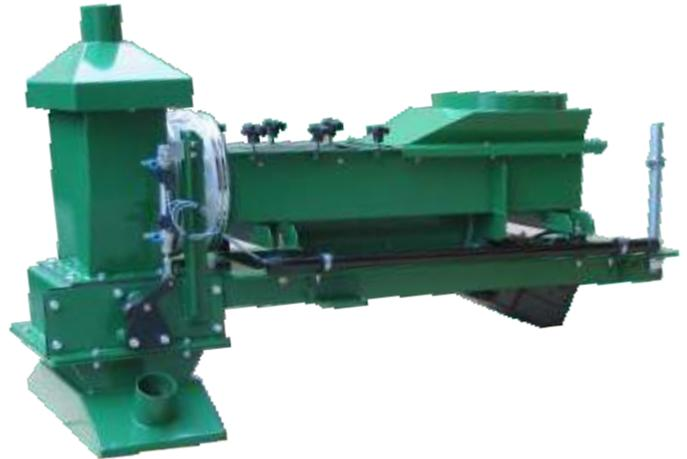
Vibratory systems can also be used to dispense materials from bulk hoppers and can be fitted with manual or automated depth regulation systems to provide a controlled throughput.
