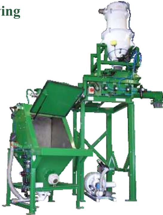
Vacuum transfer systems generally utilise rotary valves or similar feeding system to control the flow of material into the line and normally incorporate a filter or cyclone unit on the receiving vessel to separate transferring air from material.
