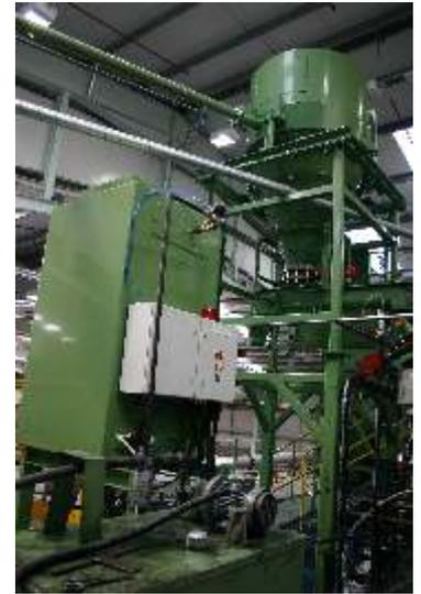
Material is transferred to the receiving vessel which is fitted with a reverse jet filtration system which separated the transferring air from the material via a series of filter cartridges. The cartridge are automatically cleaned between batches using reverse air jets.
