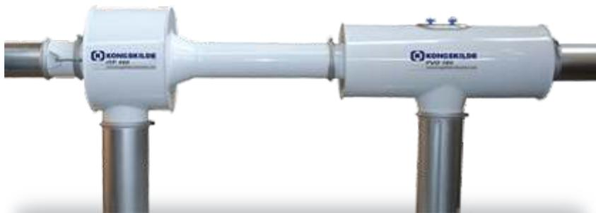
The venturi system works by creating a constriction within the pipe (classically a hourglass shape) that varies the flow characteristics of the gas travelling through the tube. As the velocity in the throat is increased a consequential loss in pressure occurs. This drop in pressure therefore creates a vacuum effect which can be used to draw material into the conveying pipeline. On the downstream side of the venturi unit the material is conveyed using the positive pressure air flow.
