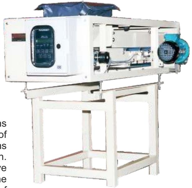
Continuous weighing systems are utilised for applications where the downstream process requires a continual feed of material rather than a batching process. Such systems generally comprise of a belt conveyor with weighed section. These weighing systems can either be used to simply give a running total of the amount of product passing over the belt or can vary the belt speed to give a constant rate of material to the process line.
