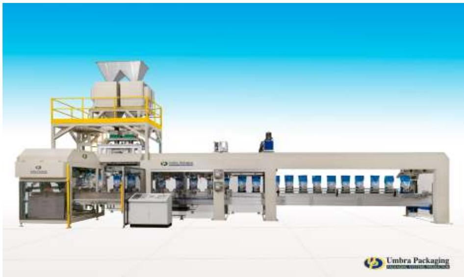
Umbra manufacture two basic lines of packaging machine; the UP1000 which handles larger format bags from 1 to 30Kg and the UP-Mini which handles smaller pack sizes from 300g to 5Kg. Both machines are available with a number of options to suit the customer's specific requirements such as:
