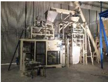
multi station filling lines with automated neck sealing, dosing, weighing and transfer mechanism we can supply a filling solution to suit you bulk packing requirements.
