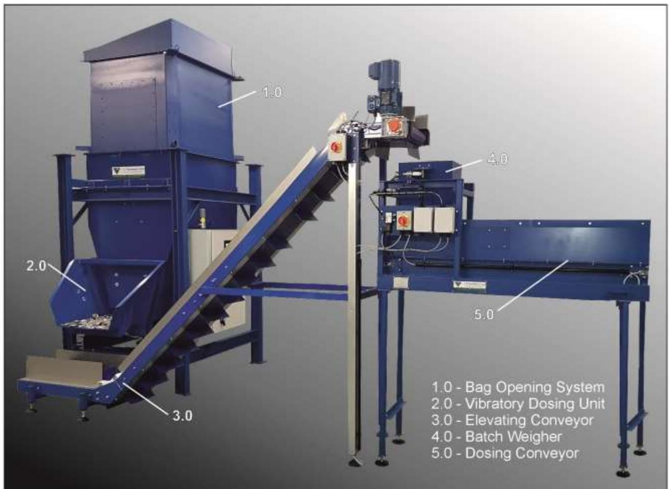
These individual machine components combine to provide an integrated turn-key solution to the customers specific requirement and are detailed in the following sections:
