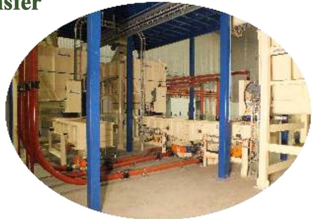
Raw materials supplied by tanker are stored in two bulk silos located outside adjacent to the building. Bulk bag materials are handled by three FIBC discharge stations with overhead gantry and power hoist system and sack materials are fed into the system via either the Comav automated sack emptying machine or via the manual sack tip station.
