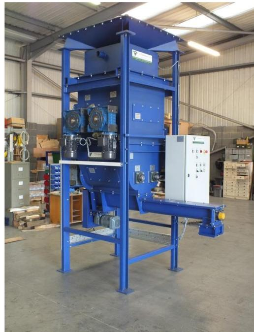
The resultant machine comprises of four elements and is designed to accept a bulk bag of material and dispense a sieved, blended product to the operator.
