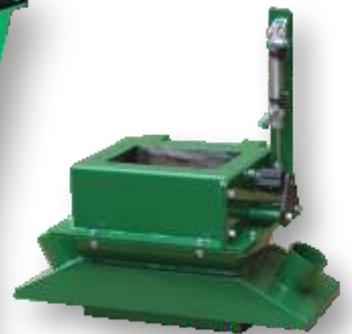
For applications where higher batch sizes and varying throughputs are required specialist feeders can be supplied which include duplex flights of different diameters to increase throughput range whilst maintaining accuracy. For maximum throughput both flights are run simultaneously and for maximum accuracy just the smaller flight is run.
