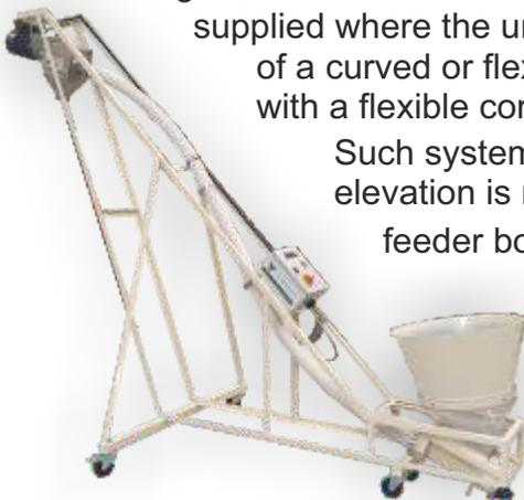
Single or twin helix agitators are incorporated for difficult materials to reduce bridging and promote a constant flow of material to the feeder flight.
