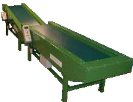
Solid material batch weighing systems generally comprise of a belt conveyor mounted on a multi-point weigh frame and provide weighing and transfer of batches to the downstream process. Loading can be performed either manually by the operator or via an automated conveyor system.
