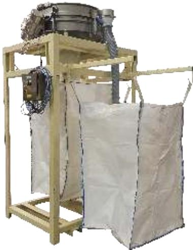
Such systems incorporate high accuracy multi-point loadcell weighing for precise filling. FIBC filling stations can be supplied for single size bulk bags or to cover a range of bag heights and can incorporate either manual or automated height adjustment dependant upon your requirement.
