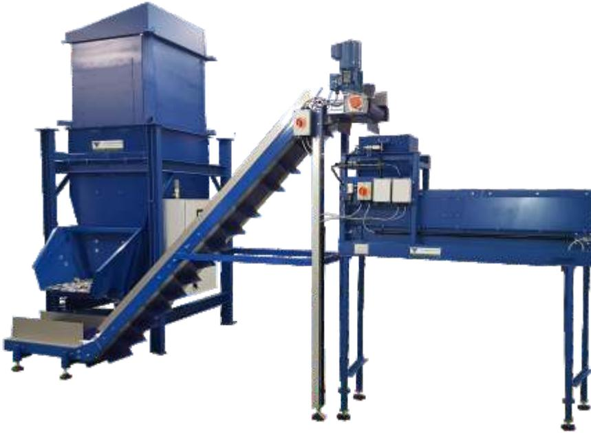
CJ Waterhouse company were initially approached to develop a bespoke dosing system for an aluminium recycling plant in Damam, Saudi Arabia. The end customer, Alcoa provided us with a brief to design a system to accurately dose aluminium can lids from a bulk bag source into the downstream process line at varying rates from 20 – 80Kg/hour.
