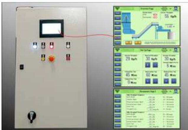
The machine mounted control panel houses a block PLC which provides sequence control of the can lid dosing system. The panel also incorporates a door mounted HMI unit providing a graphical representation of the system together with numerous data presentation, set up and configuration pages.
