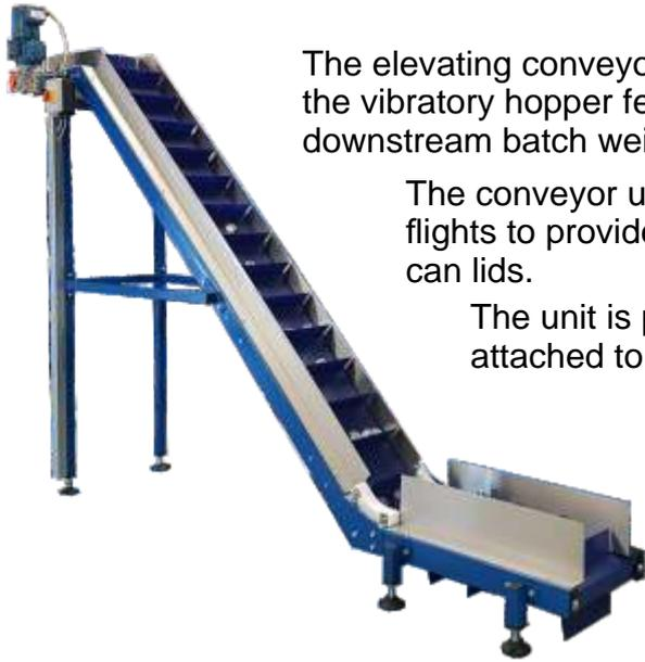
The elevating conveyor collects the can lids from the discharge point of the vibratory hopper feeder and is designed to deliver them to the downstream batch weigher at a controlled rate.
