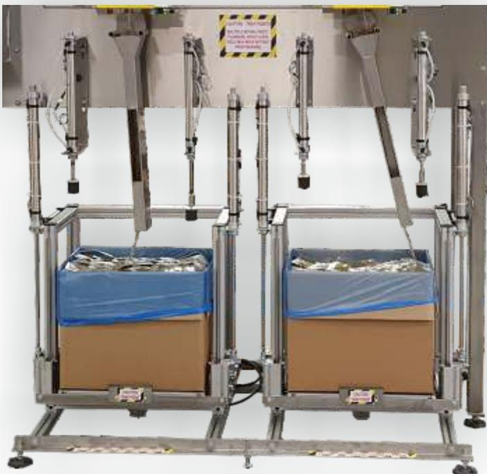
The boxes are located upon a moving carriage system, as the chute swings across the box width the carriage moves backwards and forwards at a constant rate to provide an evenly distributed layer of sachets within the box.
